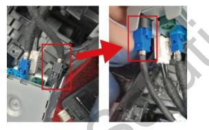
6. Connect camera to camera inputs harness, and finish installation.
