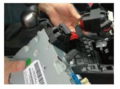
5. Factory LVDS, from main unit to Interface box; Interface LVDS, from Interface box to Factory LVDS postion;
