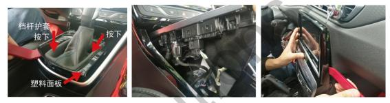
2. Be aware of screws marked on the pictures. (Around LCD, Center console and GearBox.)
