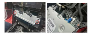
4. Plug out of Quadlock connector, and connect it to Interface cable accordingly.
